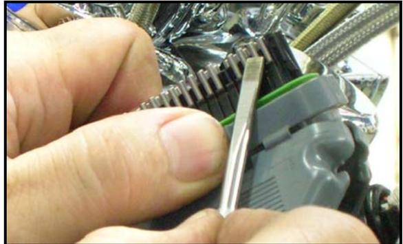
**6.** Re-install the connector retainer. Position the wires of the pigtail harness so that they exit the strain relief along the same path as the OEM wires. Close the halves of the strain relief around all wires.
