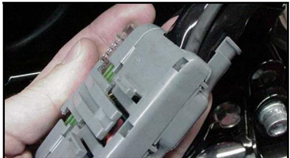
**7.** You can now position the Pigtail cable for easy access to your computer cable. Use the provided rubber dust cap to protect the open end of the mini USB Pigtail while not in use.
