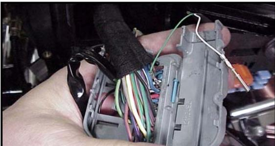
**4.** Locate the black (some models black/green) wire in port #10 (this is a redundant ground wire in the stock harness). Remove the pin & wire from #10. Insert the pigtail's terminated black wire into pin 10 on the "wire side" of the connector. Pull the stock harness's wire back to cover with provided heat shrink and tuck into wire loom.
