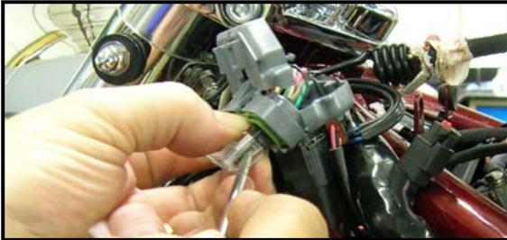
**3.** Locate the blue seal pins in unused ports #16 & #32. Remove the seal pin plugs from #16 & #32 (push out from terminal side with pick). Insert the terminated green wire into pin 32, and the white wire into pin 16 on the "wire side" of the connector.
